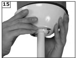
Next lift the canopy, twist into place and tighten 2 screws securely. The canopy should adjust for any irregularity in the ceiling or Outlet box.
